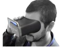
and iris recognition verifies the user's identity so the system can be used remotely without supervision. A software dashboard controls testing schedules. Results are displayed on the smartphone and the software dashboard. The SOBEREYE system provides a quick way to evaluate impairment risk, particularly when sleep disorders, alcohol or drugs are combined with fatigue.
